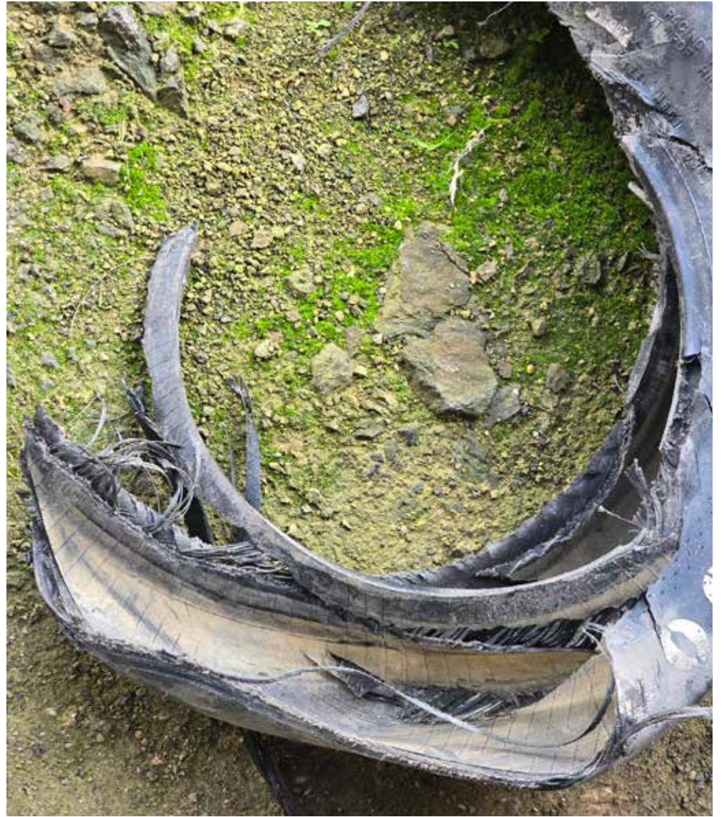
Right: This tyre exploded after it reached a speed of 536 miles per hour on a testing machine, shredding Reg Cook's attempt to break a world land speed record.
